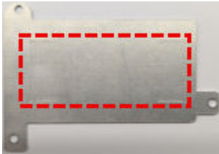
Figure 2-15 Thermal pad attached to the heatsink
