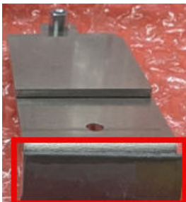
Figure 2-19 Thermal pad attached to the heatsink-2
