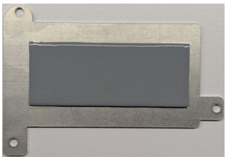
Figure 2-15 Thermal pad attached to the heatsink
