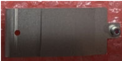
Figure 2-18 Thermal pad attached to the heatsink-1
