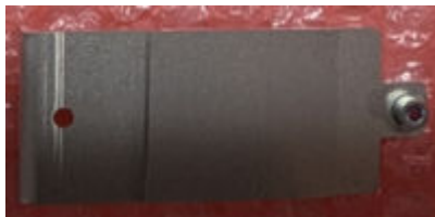
Figure 2-18 Thermal pad attached to the heatsink-1
