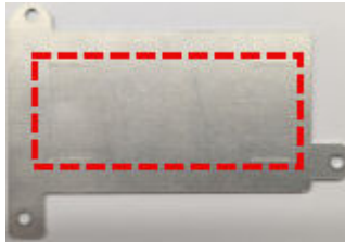
Figure 2-15 Thermal pad attached to the heatsink
