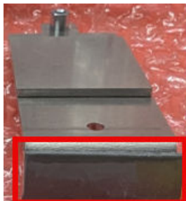
Figure 2-19 Thermal pad attached to the heatsink-2
