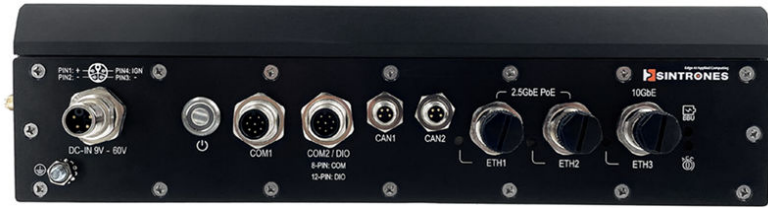
Figure 1-1 Front View of the System
