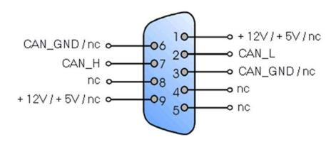
Pin assignement according to CiA recommendations DS102-1. The CANUSB is powered from USB port, so no need to connect external power on pin 9. Use only CAN\_L (pin2), CAN\_H (Pin7) and CAN\_GND (pin3).
